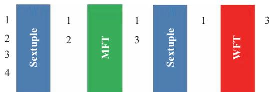
Fig. 7 (color online) An illustrative diagram for the production of the polarized hydrogen atomic beams. Two sets of sextuple magnets are used to filter out the Zeeman states |3⟩ and |4⟩ with negative electron spin. The rf transitions MFT and WFT are adjusted to induce interchanges  $2 \leftrightarrow 3$  and  $1 \leftrightarrow 3$ . Nuclear polarizations +1 and –1 can be selected by switching the WFT.
