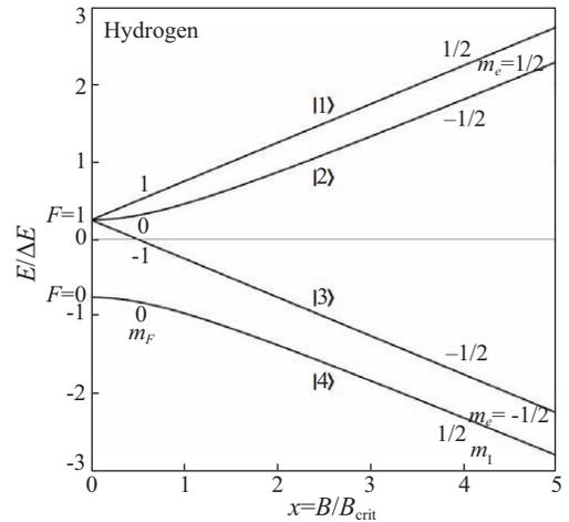
Fig. 3 The Breit-Rabi diagram of the hydrogen atom. The magnetic field and the energy are normalized by the critic field  $B_{\text{crit}} = 50.7$  mT and the hyperfine splitting energy  $\Delta E = 5.87 \times 10^{-6}$  eV.
