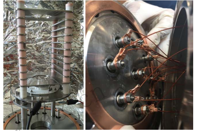
Fig. 6 (color online) Enameled wires for each bias electrode (left) and 18 bias electrodes connected to 9 feedthroughs (right).
